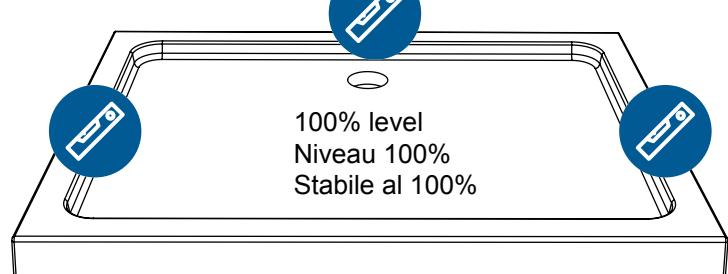
If installed on the shower tray - The tray must be fitted level, tiled in and sealed along its entire wall length.
